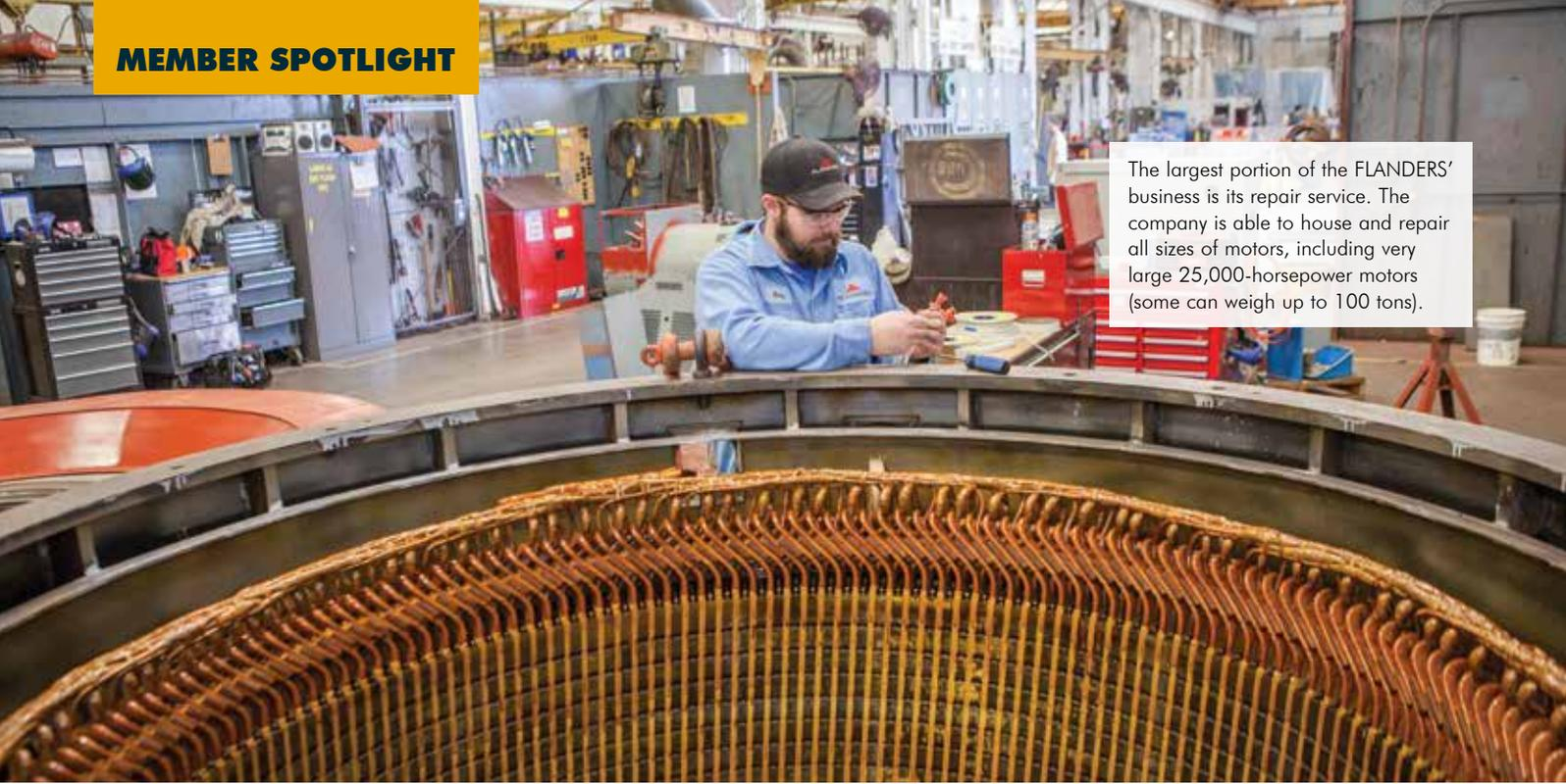
The largest portion of the FLANDERS' business is its repair service. The company is able to house and repair all sizes of motors, including very large 25,000-horsepower motors (some can weigh up to 100 tons).
