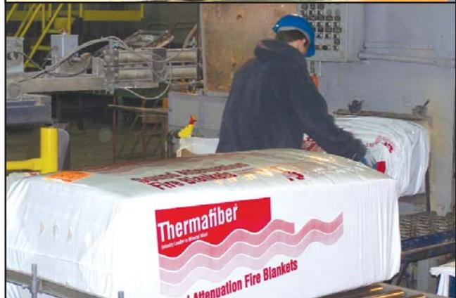
**Production process:** Thermafiber heats slag in a furnace, producing molten lava, which is spun into fiber and has a cotton candy-like texture. After treatment in a curing oven, the material can be cut into different shapes and sizes before being packaged for customers.
