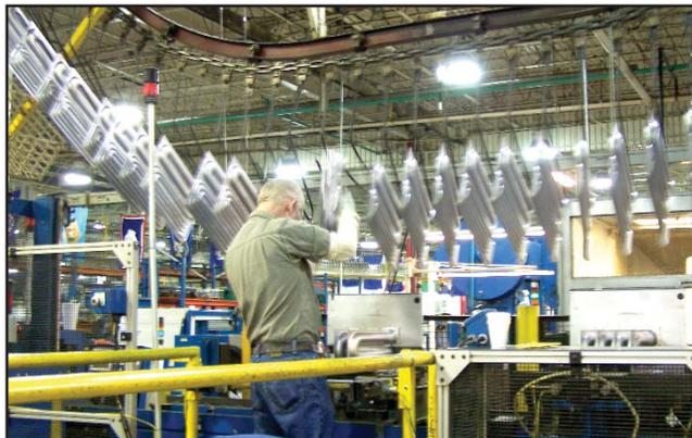
A Carrier employee places heat exchangers into a furnace unit. Heat exchangers extract heat from the ignited natural gas flowing through them to warm the home.
