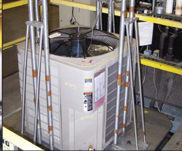
All Carrier equipment is weather-tested in a corrosion testing chamber (left) with saltwater to ensure the highest reliability and quality. This trade certified sound room (center) was built in the 1970s. It has its own foundation isolated from the rest of the building. The room, known as a reverberation room, is used to generate sound ratings for outdoor units. The shaker table (right) simulates transport of equipment to assist in packaging design and development.
