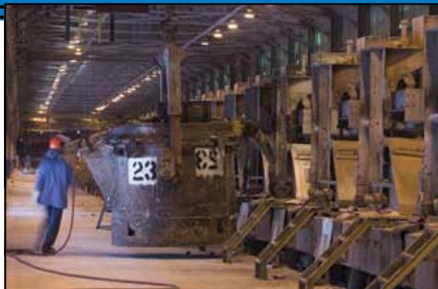
**The potrooms are the heart of the smelting process, producing molten aluminum.**
