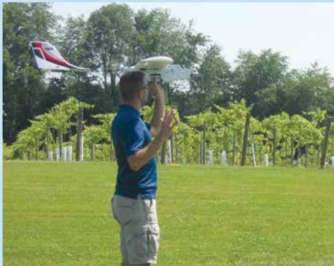
It doesn't take advanced training to get an unmanned aerial vehicle off the ground – it can be as simple as throwing it like a paper plane.
