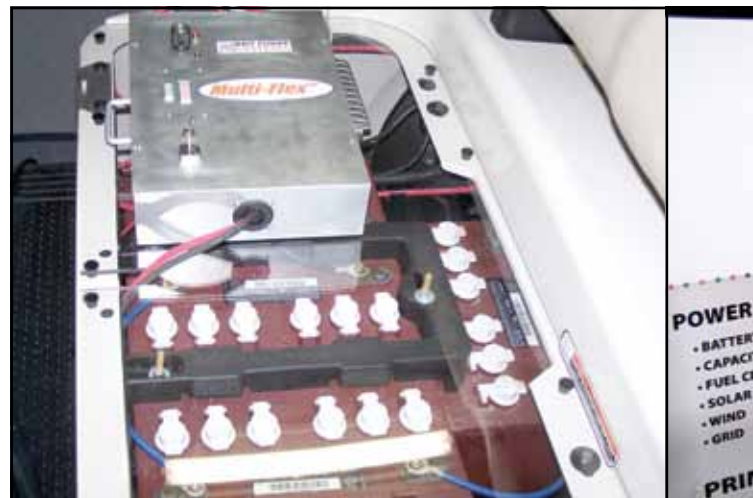
Next up is a production version of the Multi-Flex™ energy management system.
