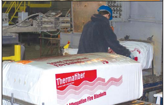
Production process: Thermafiber heats slag in a furnace, producing molten lava, which is spun into fiber and has a cotton candy-like texture. After treatment in a curing oven, the material can be cut into different shapes and sizes before being packaged for customers.
