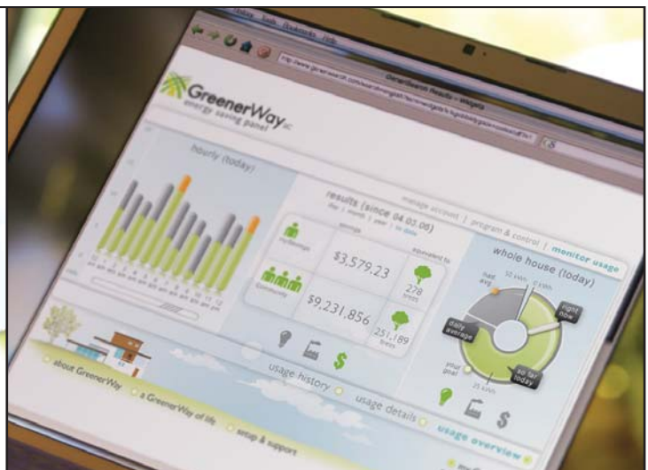
The GreenerWay system allows homeowners to monitor in real time how much energy each outlet is using. GreenerWay customers will use a web-based program to track current energy usage as well as compare day-to-day and month-to-month data.
