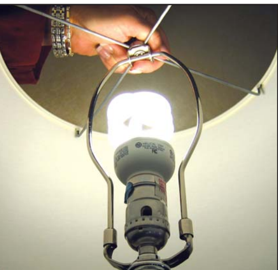
The average lifespan of a compact fluorescent light bulb is 10,000 hours compared to 750-1,000 hours for incandescent bulbs.
